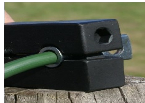
Now place the slug between the jaws of the crimper
