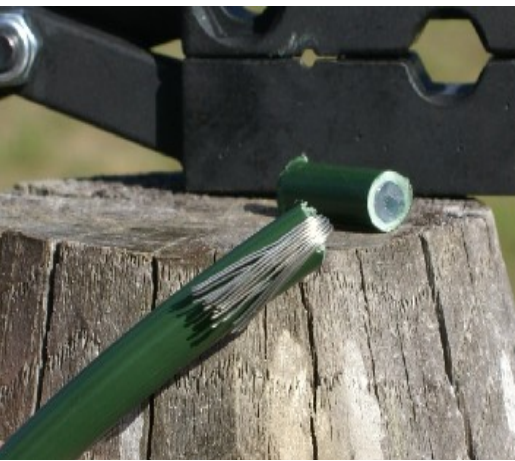
Press the harness of wires so they can slip intirely into the slug Force the cable totaly in
