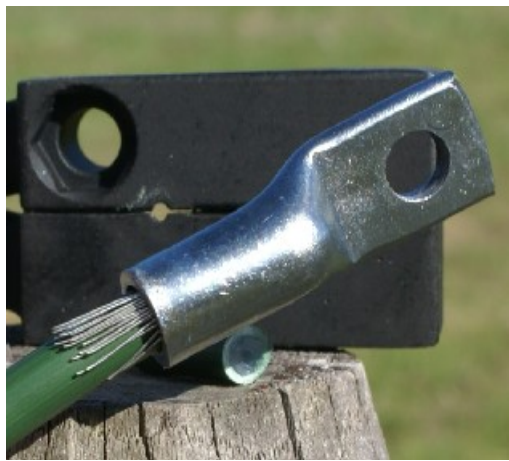
Press the harness of wires so they can slip intirely into the slug Force the cable totaly in
